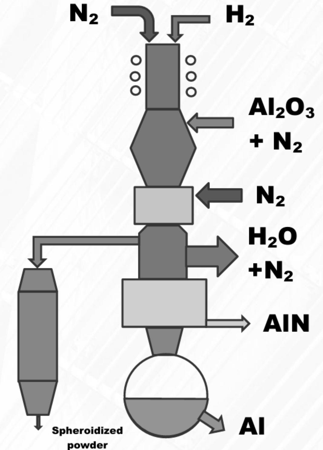
Operation at elevated pressure (up to ~5 bar) enables kinetics and control; direct molten Al feed to furnace reduces remelt losses.
