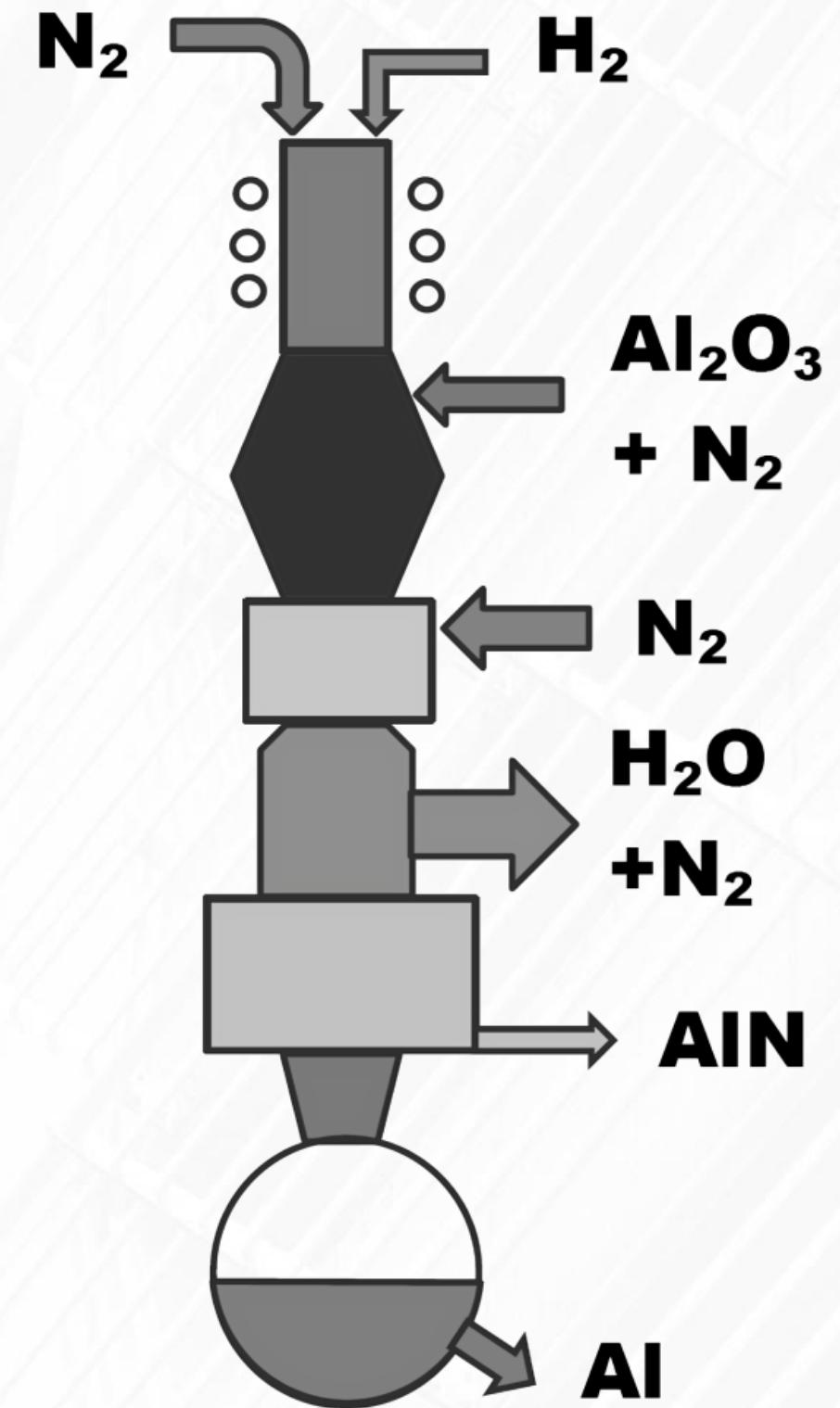
Operation at elevated pressure (up to ~5 bar) enables kinetics and control; direct molten Al feed to furnace reduces remelt losses.
