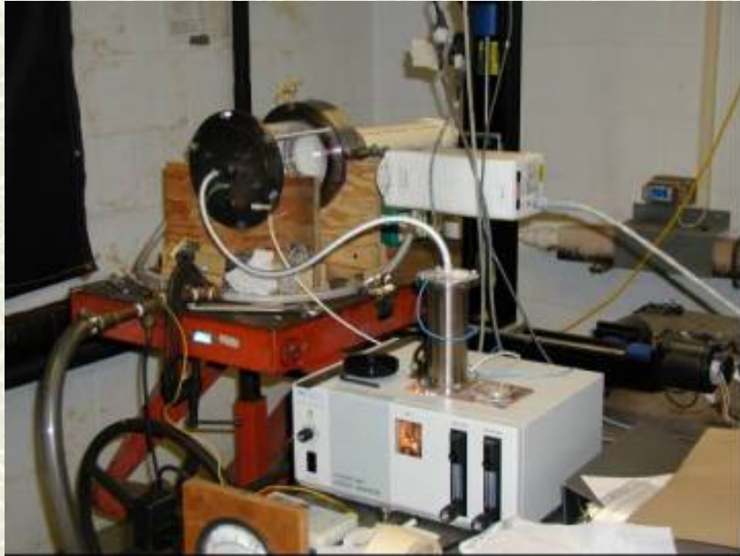
The Tornado Combustor, the LDV probe, the particle generator, and the traversing mechanism
