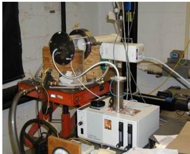
Figure 1. Experimental setup showing the plasma chamber, the LDV probe, the particle generator, and the traversing mechanism.
