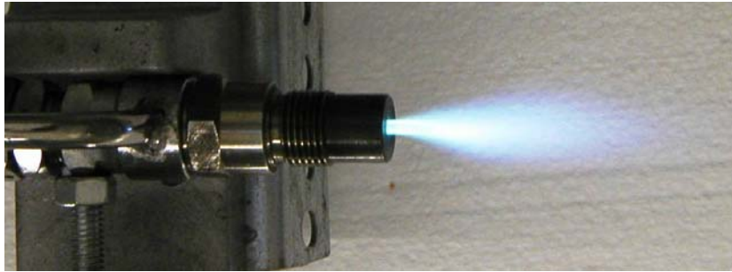
Fig.2. CCPT with fuel feeding into the arc chamber in operation.
