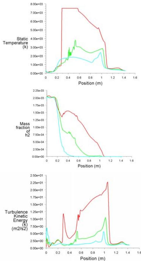
Fig. 7. Dependences of static temperature, mass fraction of  $H_2$ , and turbulence kinetic energy on the combustor length:
