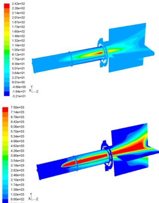
Fig. 5. Contours of mean axial velocity (m/s) and temperature (K) in a plasma torch with reverse vortex.
