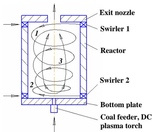
Fig. 2. Flow schematic inside the reactor.
