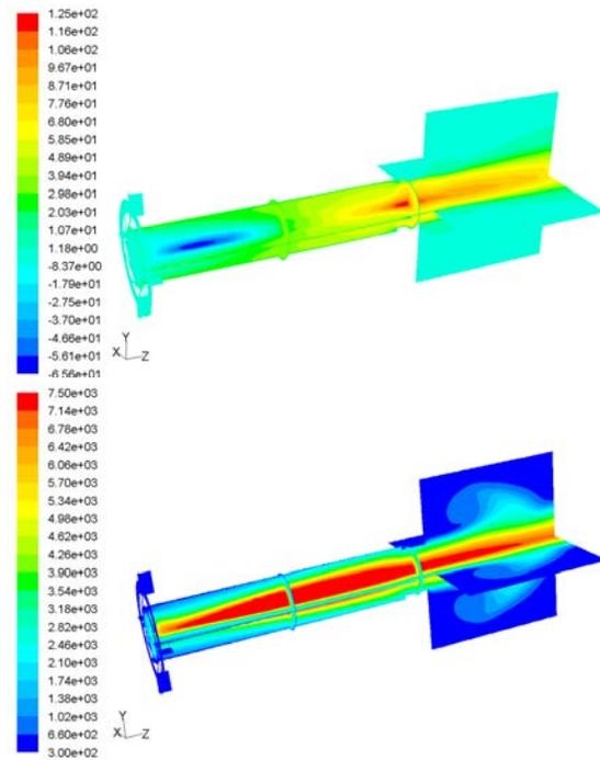
Fig. 4. Contours of mean axial velocity (m/s) and temperature (K) in a plasma torch with direct vortex.
