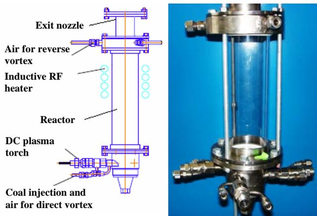
Fig. 1. Diagram and picture of the triple vortex plasma reformer.
