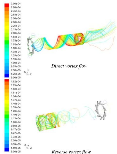
Fig. 6. Particle traces colored by particle diameter.
