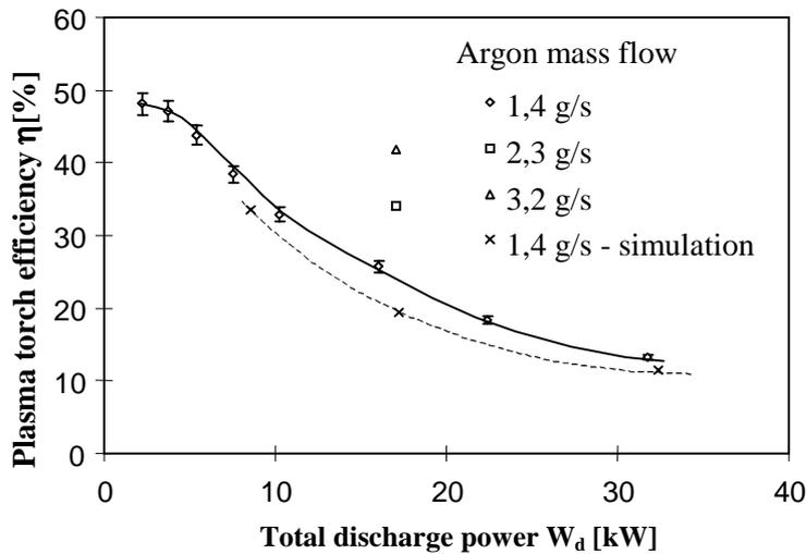
Fig. 4. Argon FVS ICP. Dependence of the plasma torch efficiency on the total discharge power for different argon mass flow. Experimental and simulation.
