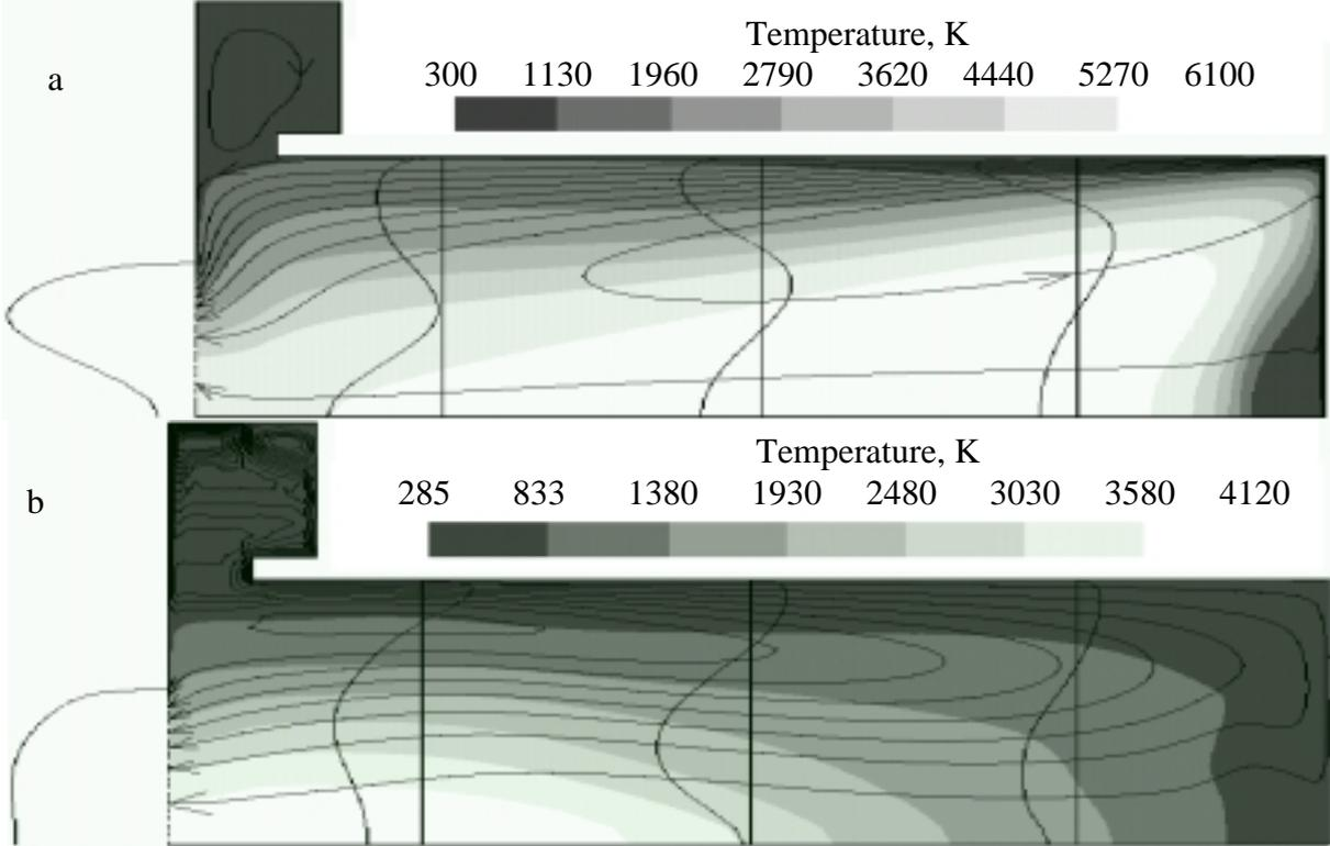
Fig. 2. Modelling results for MW plasma torch.
