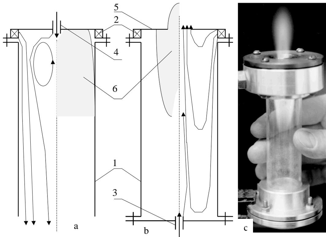
Fig. 6. Schemes and picture of the gas burners of 2 kW power.
