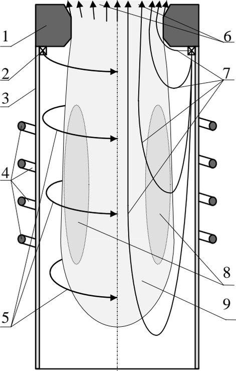
Fig. 3. Scheme of the inductively coupled RF plasma torch with RVS.
