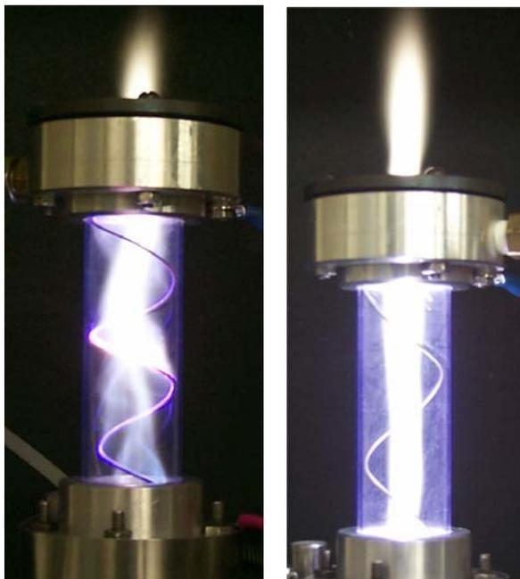
Figure 8: Tornado Gliding Arc (left) may transform to the high voltage atmospheric pressure discharge inside the Reverse Vortex Flow (right).
