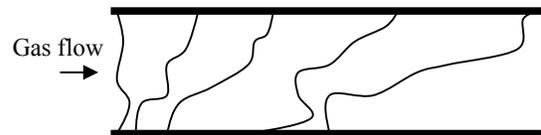
Figure 7: Elongation of arc on parallel electrodes but with different gas flow velocities near the two electrodes
