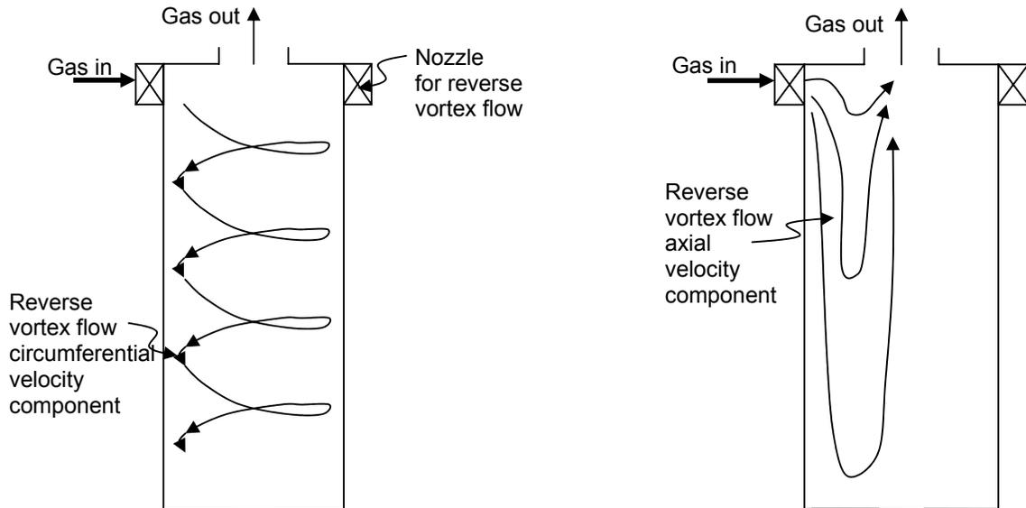
Figure 1: Reverse Vortex (“Tornado”) flow in a cylindrical reactor.
