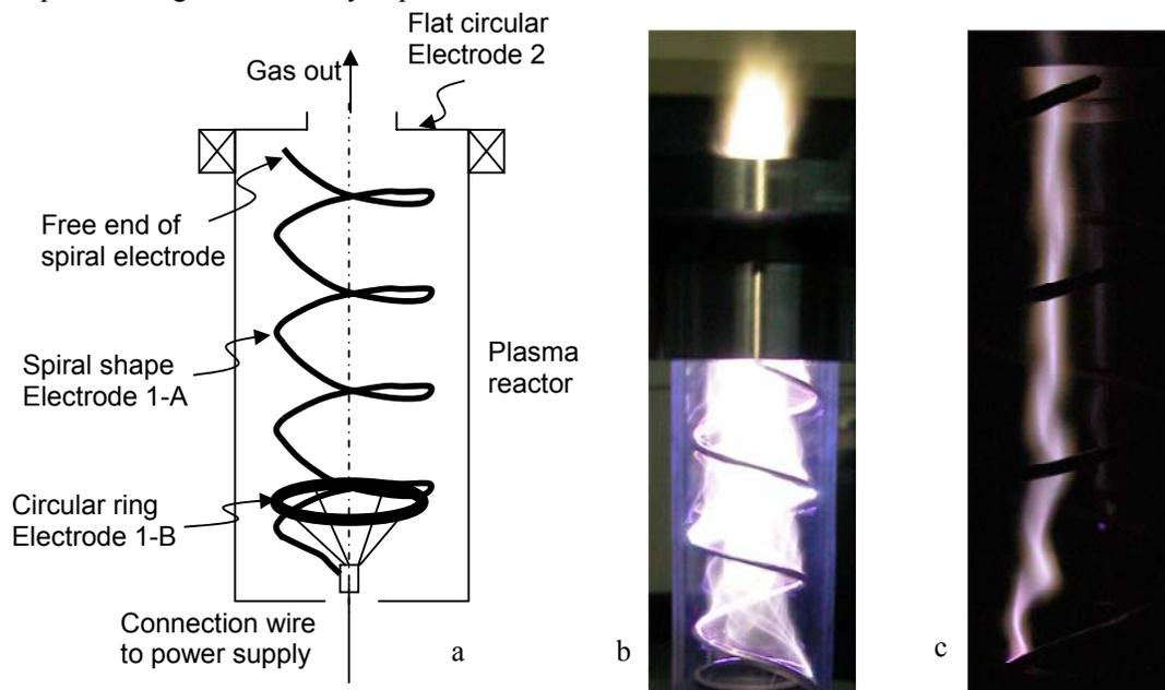
Figure 5: Tornado Gliding Arc (TGA), a – schematic of TGA reactor; b - photo image of gliding arc with normal exposition time; c - photo image of gliding arc with shot exposition time (1/1000 s).
