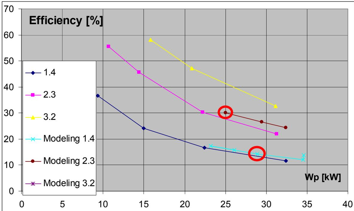
Figure 3: Comparison between the experimental data [9] and simulation for three levels of argon flow rate 1.4, 2.3 and 3.2 g/s. Red circles mark the points presented in Fig. 4.
