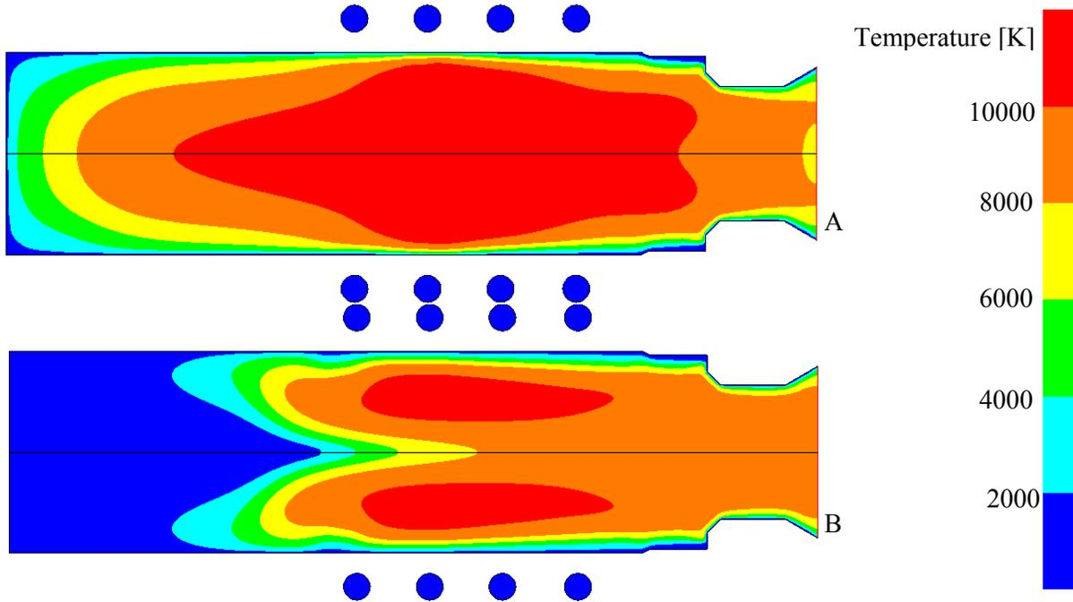
Figure 4: Temperature field for two simulated cases marked by red circles in Fig. 3: (A) – 1.4 g/s of argon and 28 kW of plasma power; (B) – 2.3 g/s of argon and 25 kW of plasma power.
