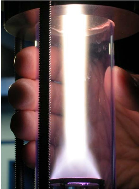
Figure 6: Tornado Gliding Arc (TGA) between circular electrode and flange (flat circular electrode).
