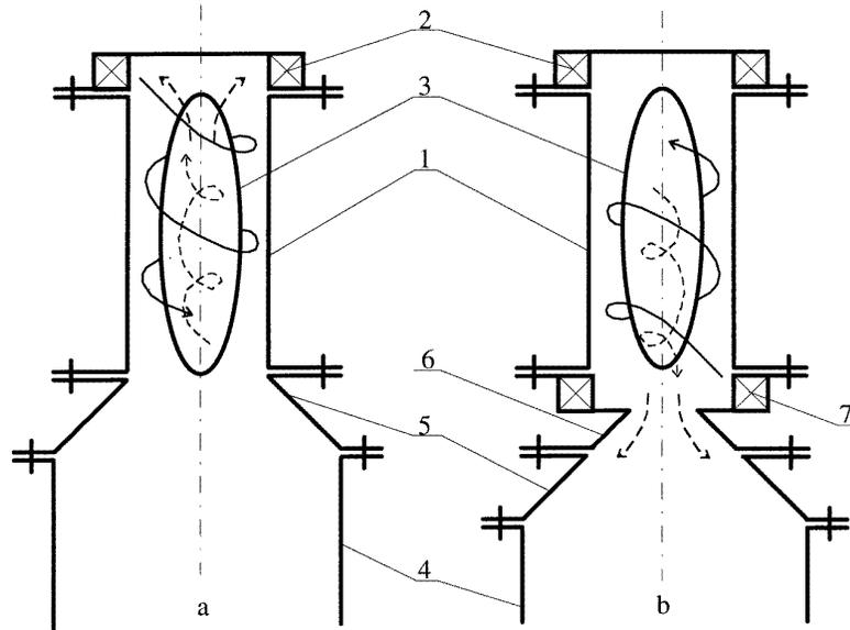
**Figure 1.** Schematic diagrams of the MW plasma torch with supposed flow patterns of gas and plasma: (a) the 'old' scheme with flow patterns for conventional vortex plasma stabilization and (b) the 'new' scheme with flow patterns for *reverse vortex* plasma stabilization.
