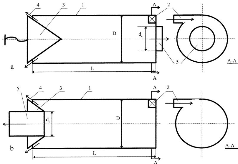
**Figure 5.** Schematic diagrams of the counterflow (a) and parallel-flow (b) vortex tubes.
