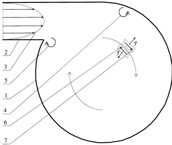
**Figure 6.** The proposed scheme of the energy separation in the vortex tube.
