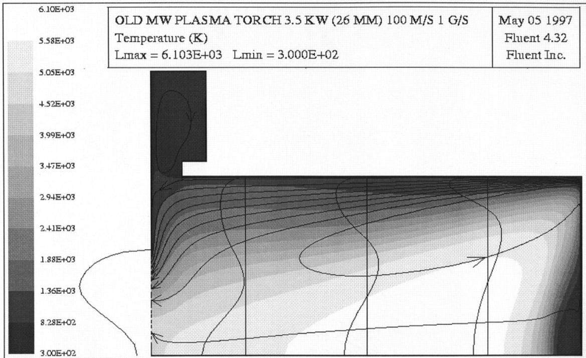
**Figure 3.** The temperature distribution, stream lines and contours of axial velocity for three different cross sections and for the outlet of the MW plasma torch with conventional vortex flow.
