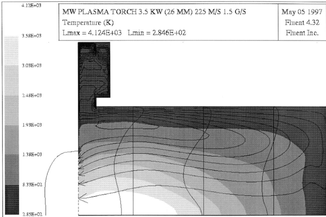
**Figure 4.** The temperature distribution, stream lines and contours of axial velocity for three different cross sections and for the outlet of the MW plasma torch with *reverse vortex flow*.
