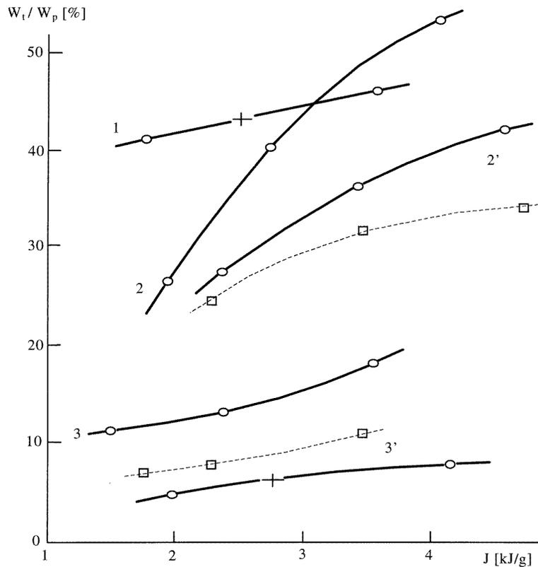
**Figure 2.** Heat losses in the microwave plasma generator: full curves, experiments; broken curves, numerical simulations.
