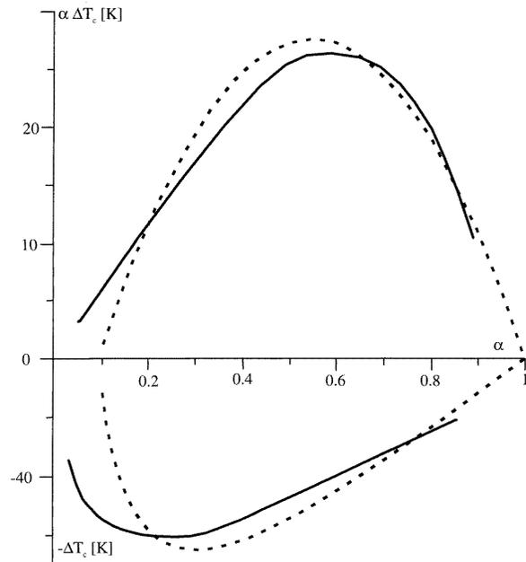
**Figure 7.** Characteristics of the vortex tube: full curves, experiment [6]; and broken curves, theoretical estimations based on the proposed model [9].
