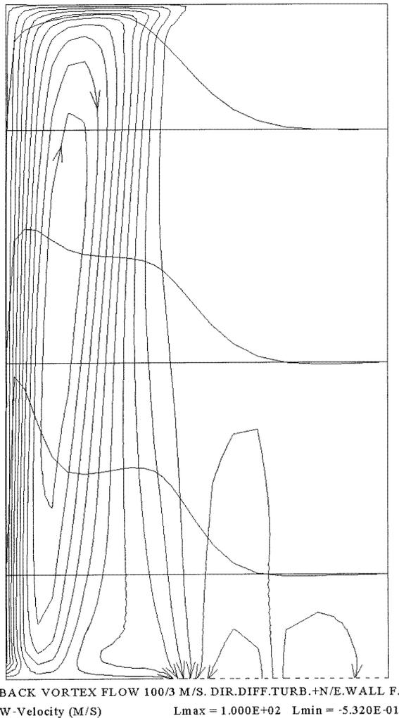
**Figure 8.** Stream lines and tangential velocity  $W$  contours for confined *reverse vortex flow*.
